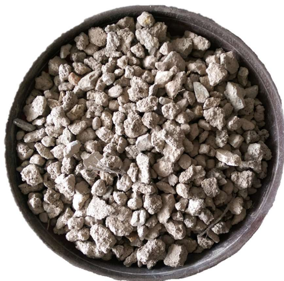
Figure 1. Recycled aggregate concrete fraction (8–16 mm).
