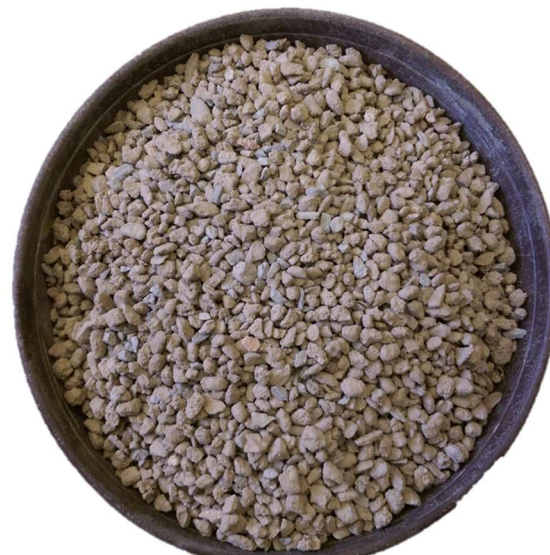
Figure 2. Recycled aggregate concrete fraction (4–8 mm).
