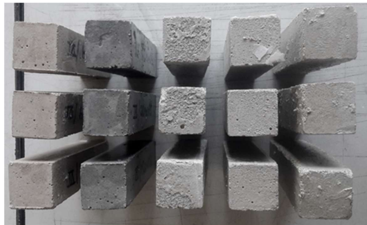
Figure 4. Photo of the gypsum-based composites and gypsum mortar stored under the water (W), 360 days old; from the left: crushed ceramic-KC, Silica fume-KM, GBS-KS, without pozzolan-K, gypsum mortar-G.
