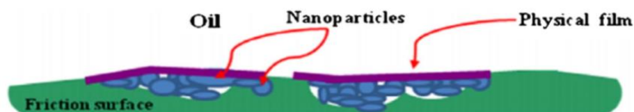
Fig. 1: Mechanism appearing how to reduce friction between oil surfaces when mixed with nanoparticles [26].
