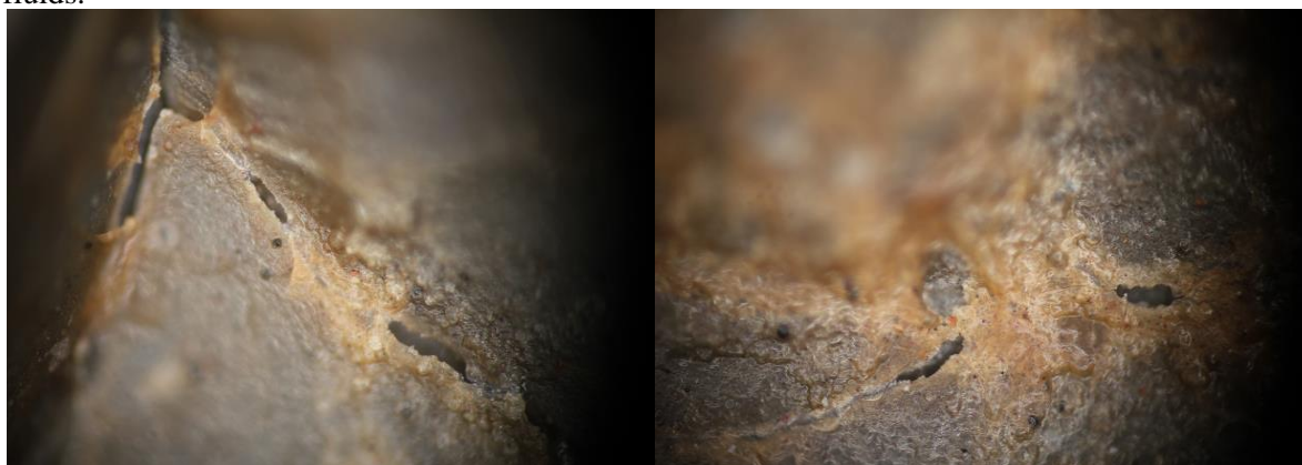
Figure 14. The Bridge of sodium silicate between the fractures.
