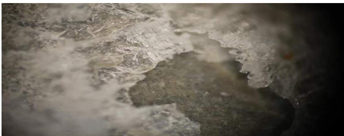
Figure 13. Crystals of the salts on the surface of the shale.
