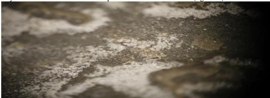
Figure 12. KCl accumulations on the surface.
