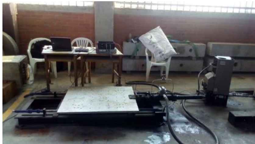
Figure 7. Experimental assembly of the hydraulic uniaxial seismic shake table.
