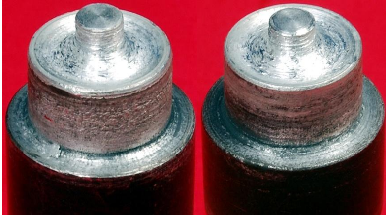
(a) Straight Cylindrical Threaded (b) Taper Cylindrical Threaded Figure 2.2 Tool Pin profiles
