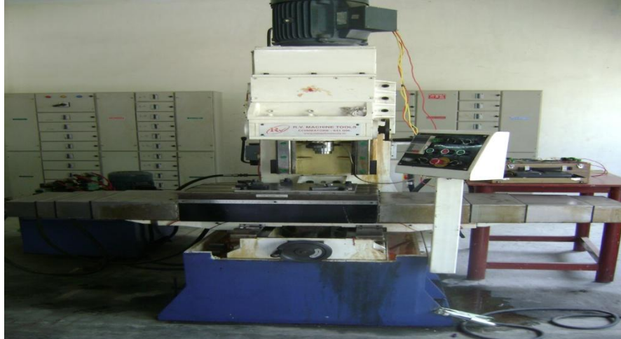
Figure 1. Friction stir welding machine
