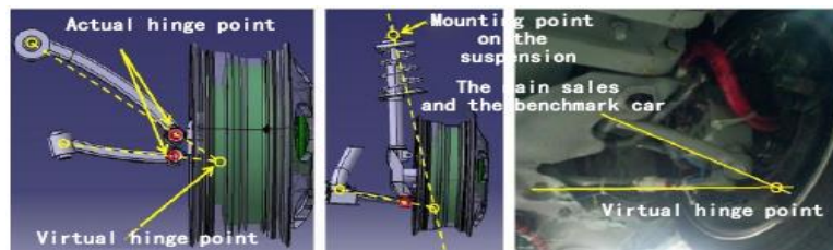
Figure 3. Double-section arm suspension and virtual hinge point
