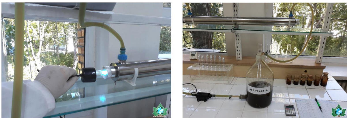
Figure 1. Experimental setup used for the UV treatment of wastewater.
