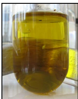
Figure 9. Acid digestion of samples in ECO6 thermoreactor - control sample .
