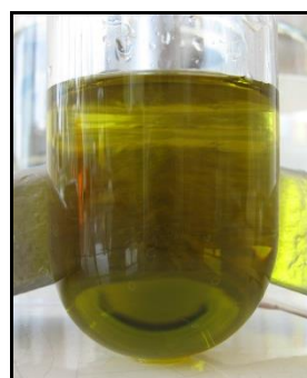
Figure 10. Acid digestion of samples in ECO6 thermoreactor - Strain sample .
