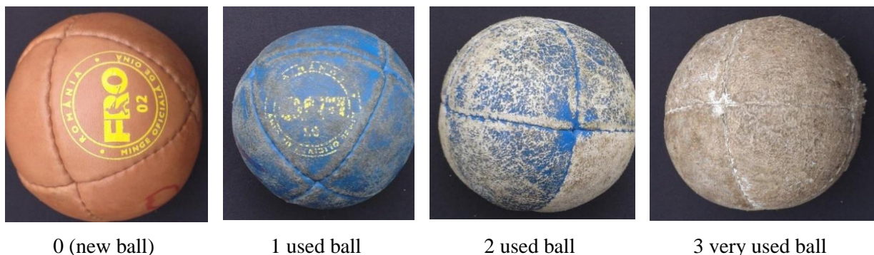
Figure 3. The 4 groups of the balls (0-new, 1,2,3very used ball), with different wear degrees.
