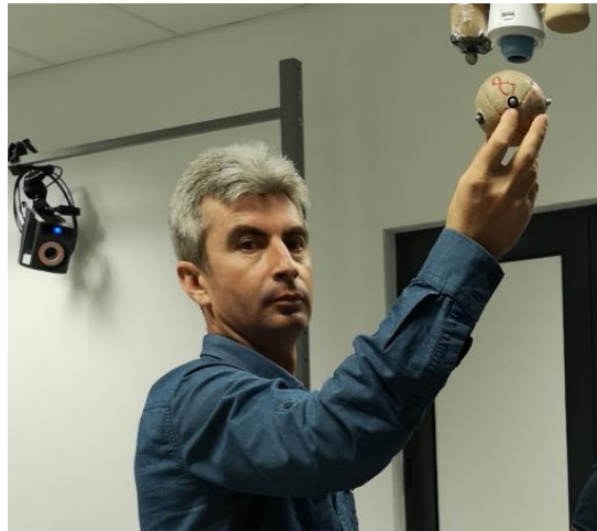
Figure 5. The oina ball with 4 markers suspended by vacuum pump.
