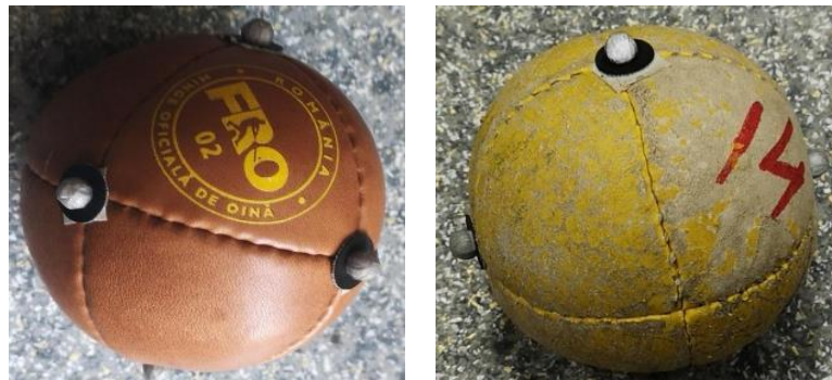
Figure 4. The oina balls (new and used) with 4 markers.
