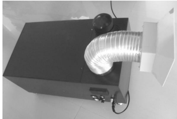
Figure 5. Dust smoke eliminator using c-ozone (corona ozone) electric energy.
