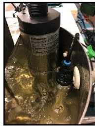
MBBR equipped with sensors for dissolved oxygen and ammonia
