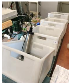
Figure 6. Tanks and biofilm carriers used to determine the efficiency of the new material.
