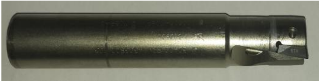
Figure 1. SECO cutting tool type R217.69-1616.0-09-2AN used to conduct experiments.
