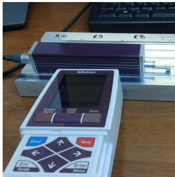
Figure 2. Making roughness measurements using the Mitutoyo SURFTEST SJ-210.
