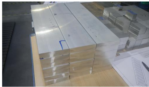
Figure 1. Preparation of the 21 Al7136 blocks to be machined.
