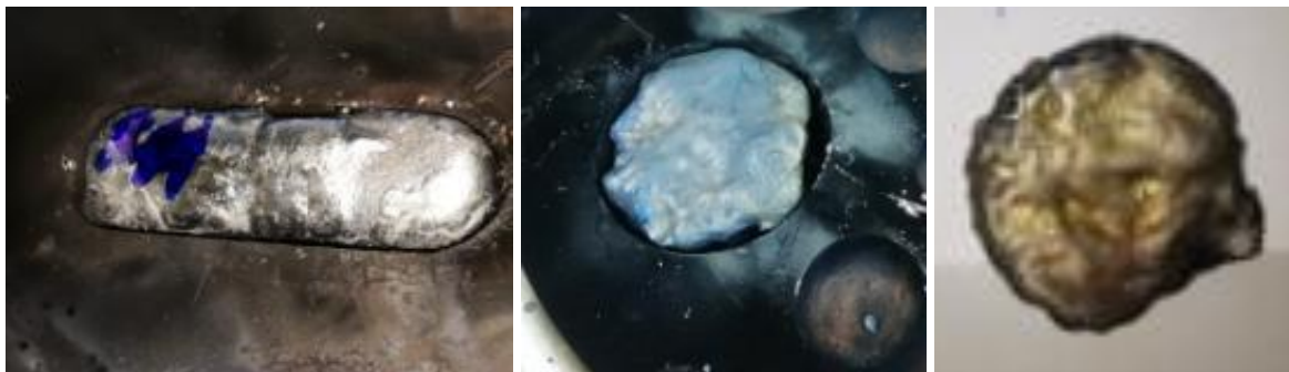
Figure 1. Buttons of heavy alloys obtained by melting in the VAR equipment.
