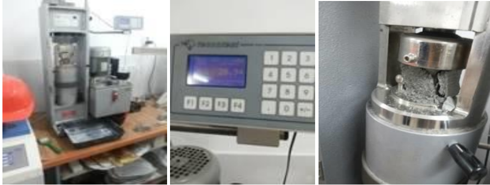
Figure 2. Testing compression strength.
