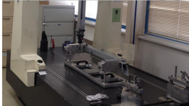
Fig. 1 a) the key indicators of the ball pin, affecting the performance of the function of official purpose, b) the IOTA 2204 measuring machine in the process of measurement. This is a rather complicated and time-consuming procedure. According to internal regulatory documents of an enterprise, 1-2 out of 100 manufactured parts are exposed to measurement. As a consequence, the rapid assessment of values for the management of these indicators in the process is impossible [2, 3].
