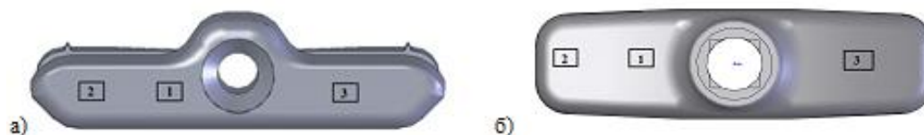
Figure 1. Determining roughness on the resulting casting and the casting of ZAMAK-5; b – casting aluminum alloy
