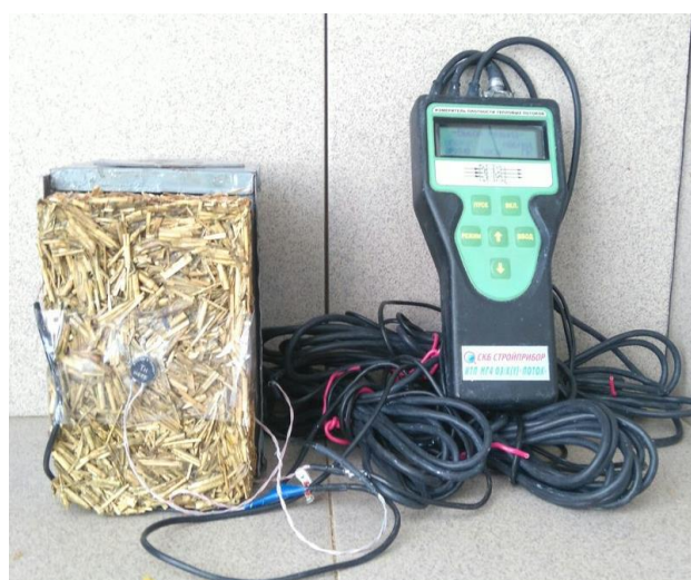
Figure 2. Air thermostat with a device ITP-MG-4.03 X(Y) «Potok».
