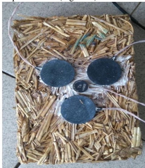
Figure 1. Straw material plate - rubber with heat flux density sensors and temperature sensor
