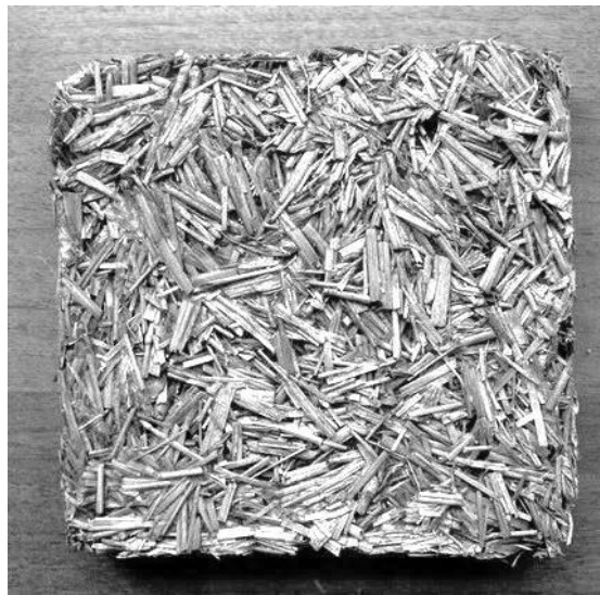
Figure 6. Sample based on straw and SKI-3 C-nitrous vulcanization rubber after exposure to the external environment for one year.
