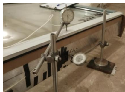
Figure 10. The area of calculated buckling of a fragment of the facade system. Installed strain gauges and dial gauges
