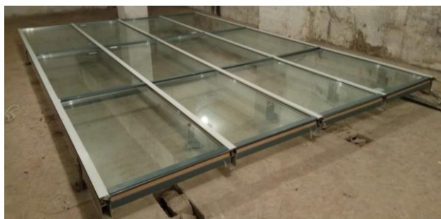
Figure 9. General view of the tested fragment of the facade system
