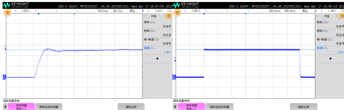
Figure 10. Variable structure high voltage power supply waveform based on predictive PI algorithm.
