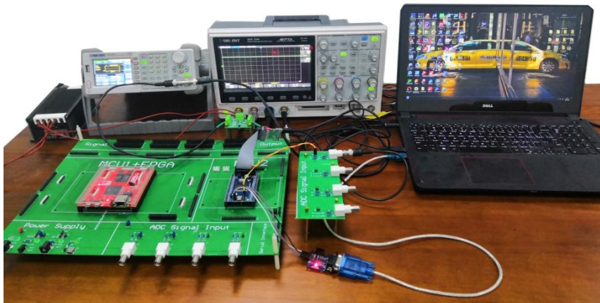
Figure 9. System experimental control platform based on ARM and FPGA architecture.
