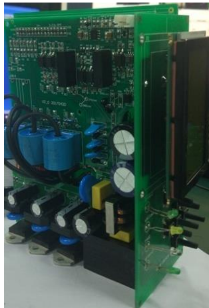
Figure 5 microcomputer relay protection device with electric-take ring
