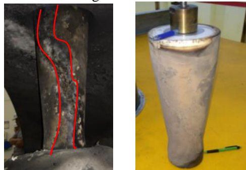
Figure 2. Particles and flashover discharge traces on supporting insulator in fault bushing
