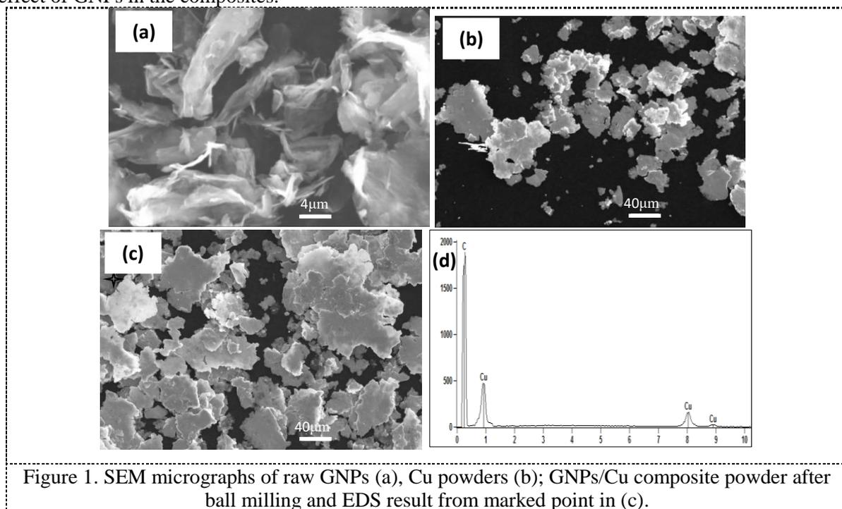
Figure 1. SEM micrographs of raw GNPs (a), Cu powders (b); GNPs/Cu composite powder after ball milling and EDS result from marked point in (c).
