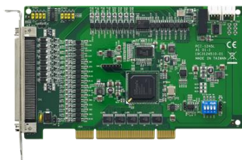
(a) Advantech PCI-1245L motion control card
