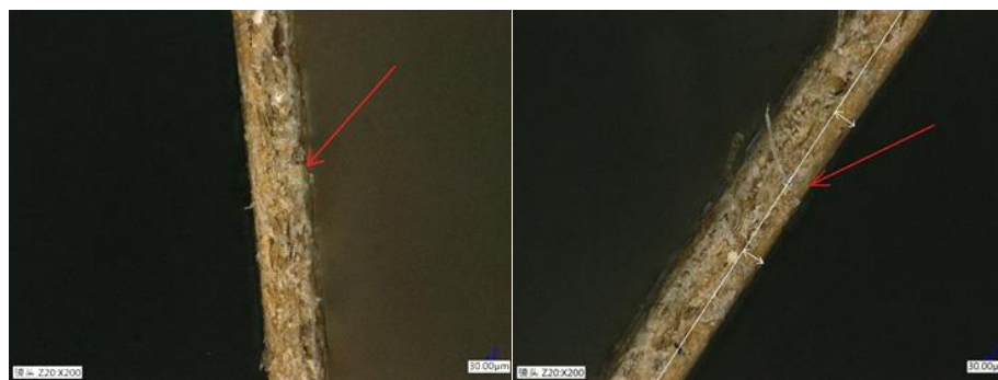
(a) cross-section of base paper (b) cross-section of coated paper
