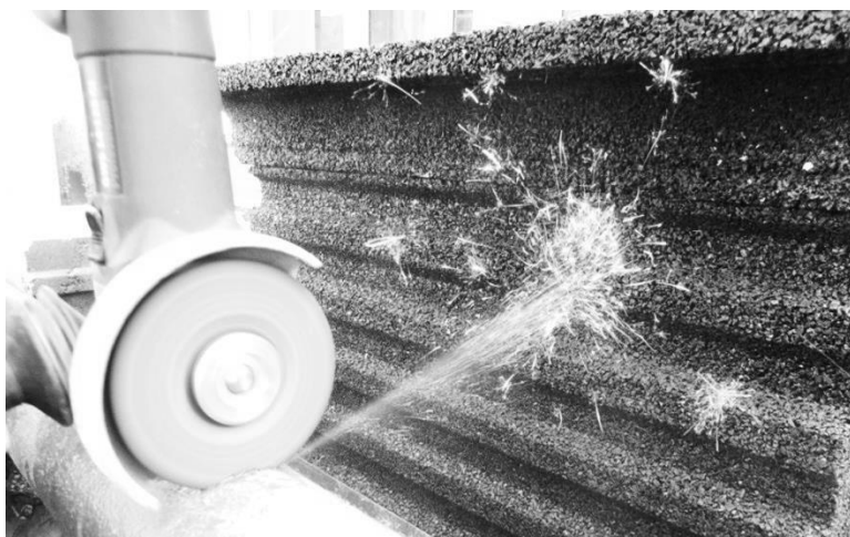
Figure 3. Test 1 - simulating rail grinding.
