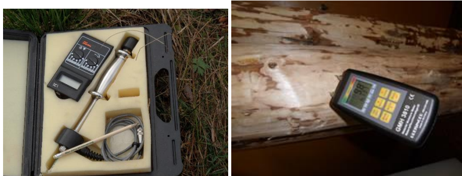
Figures 2 and 3. Hygrotest 6500 Resistance Hygrometer and Resistive Moisture Meter with GMH 3810 Integrated Probes.
