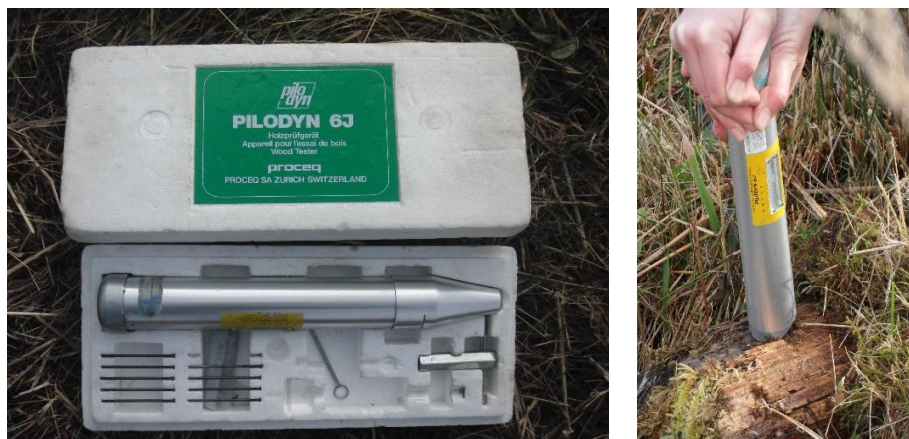
Figures 4 and 5. Pilodyn 6J Resistance Stroke Instrument - Measurement on Threshold Side Wing.
