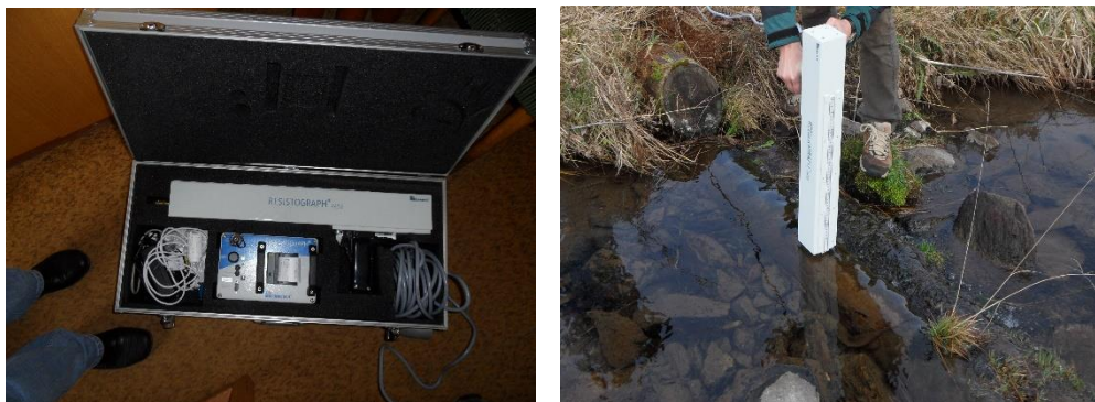
Figure 8 and 9. Resistograph 4453 Resistance Micrometer - Measurement on Overflow Edge in the Middle (Wood in Water).
