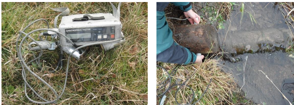
Figures 6 and 7. Non-destructive Arborsonic Decay Detector - Measurement on the sill side.
