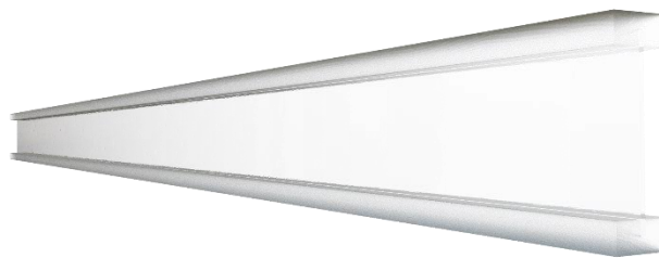
Figure 1. Transparent wood “I” beam rendering [7].
