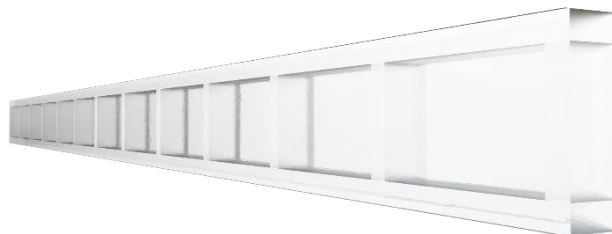
Figure 2. Transparent wood Vierendeel box beam rendering [7].
