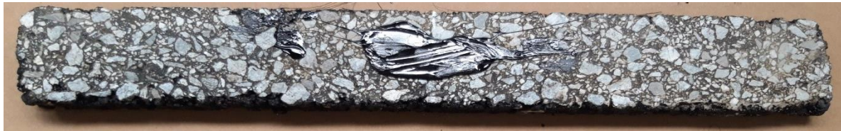
Figure 1. Direct micro wire application using bitumen on the beam (1 st test sample).
