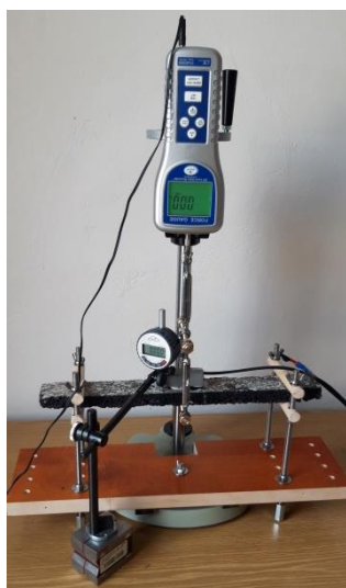
Figure 3. three-point bend with 1 st test sample.
