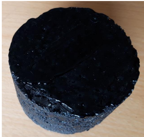
Figure 2. Direct micro wire application using bitumen on the 2 nd test sample.
