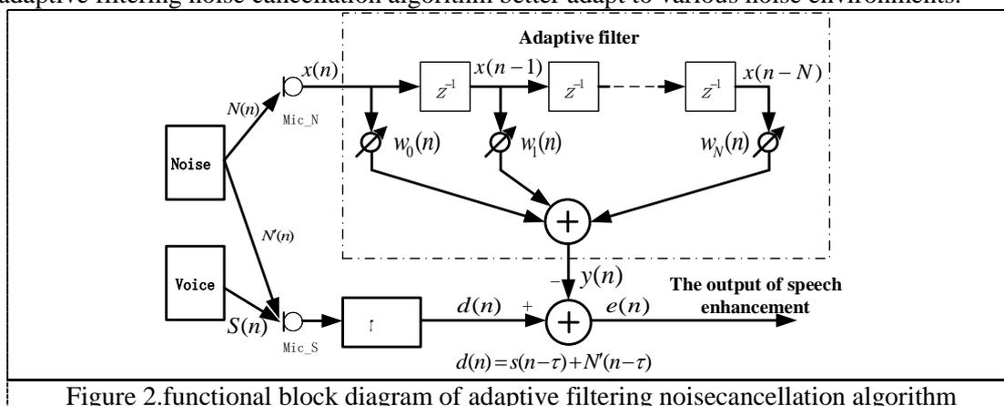
Figure 2. functional block diagram of adaptive filtering noise cancellation algorithm
