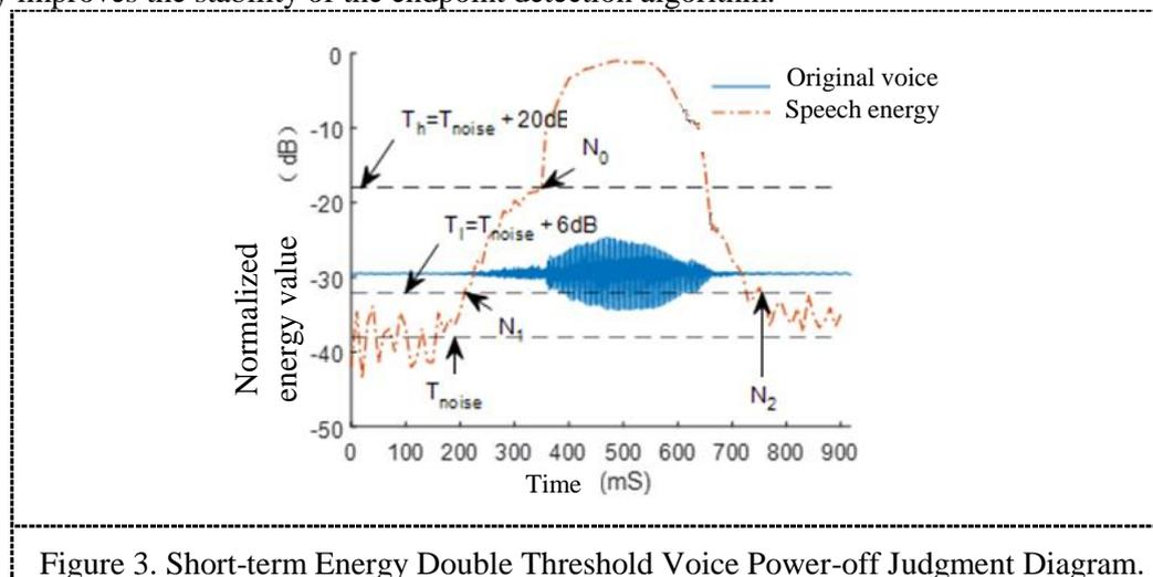
Figure 3. Short-term Energy Double Threshold Voice Power-off Judgment Diagram.
