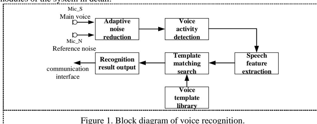
Figure 1. Block diagram of voice recognition.
