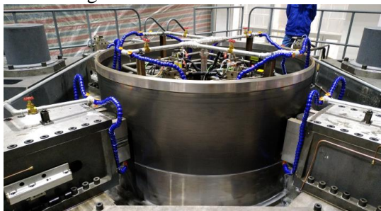
Figure 16 Counter-roller spinning experiment
