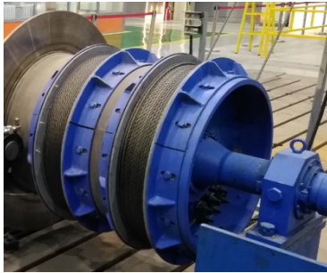
Figure 8. The winding drum of test platform.
