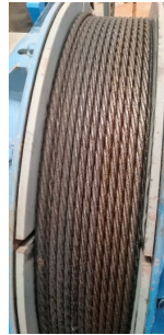
Figure 9. The normal rope arrangement of drum.
