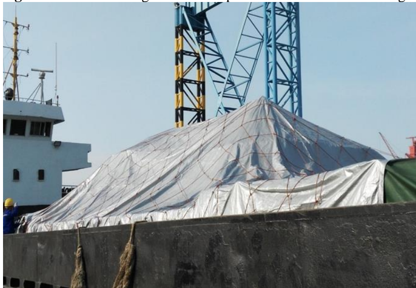
Figure 4. Schematic diagram of the cover net rope covering the tarpaulin
