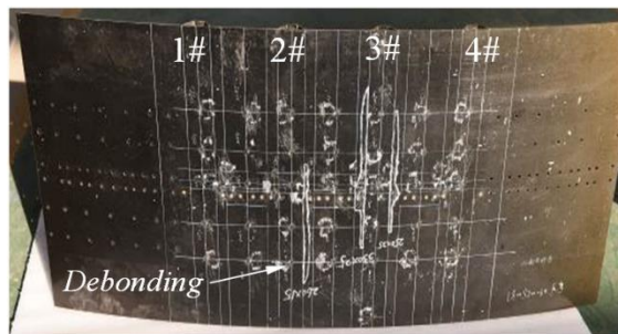
Figure 9. Debonding area of panel 1
