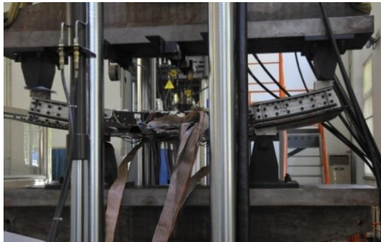
Figure 3. Four-point-bending test device
