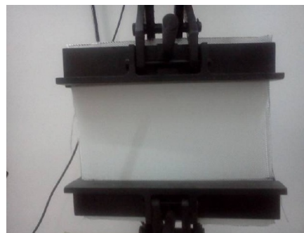
Figure 2. Tensile test of geotextiles
