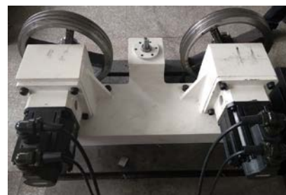
Figure 4. The novel precision gear honing machine tool transmission principle and prototype
