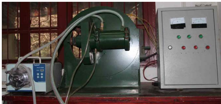
Figure 3. The preparation system for grinding submicron and nano particles via mechanical comminution.
