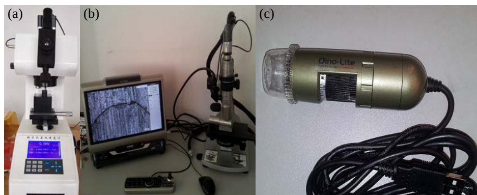
Figure 2. Measuring instruments: (a) digital micro-hardness tester, (b) VHX-2000 microscope system with super depth of field, (c) Dino-Lite portable microscope.
