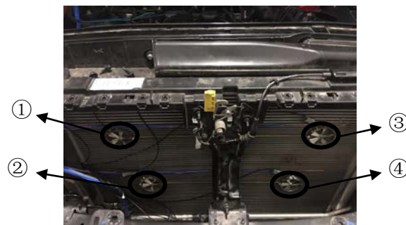
Figure 10. Flow velocity test on whole vehicle.
