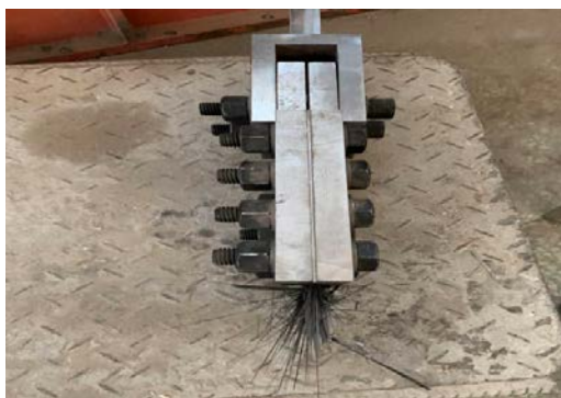
Figure 9. Carbon plate explosion damage
