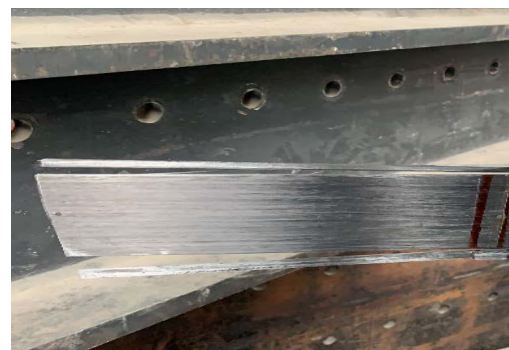
Figure 10. Carbon plate longitudinal splitting failure
