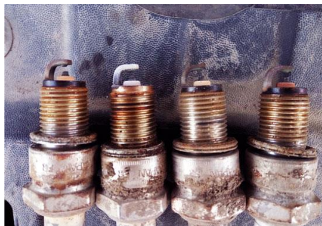
Figure 3. Faulty spark plugs.
