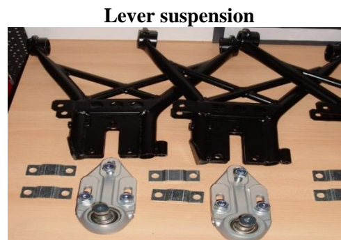
Figure 3. Reinforced tubular lever of the car suspension - Audi 90 1985.
