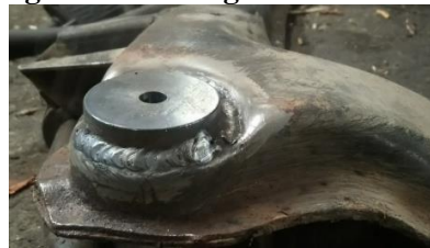
Figure 5. Steel sleeve welded to the subframe of Audi 90 1985.
