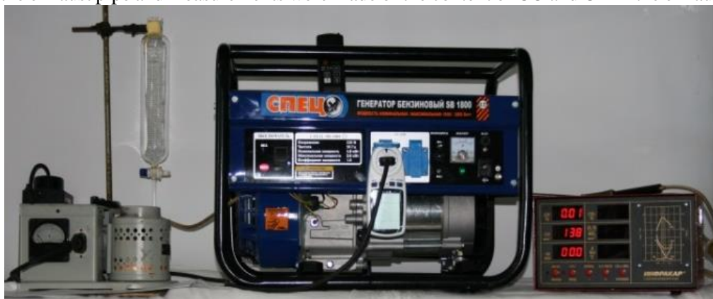
Figure 2. Test bench for motor oils.
