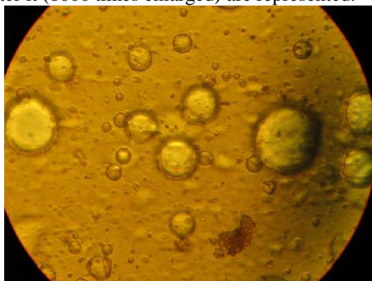
Figure 5. Experimental images of the fuel oil under the microscope (6000 times enlarged) before being treated with a disperser.
