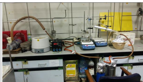
Figure 2. The experimental of vacuum distillation.
