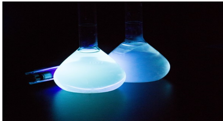
Figure 3. Developed CQD solutions showing strong blue luminescence under UV lamp
