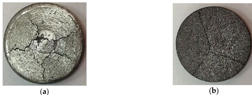
Figure 3. Character of destruction of (a) cast iron and (b) graphite discs 15 mm in diameter.
