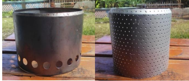
Figure 5. Air inlet at the stove wall, before modification
