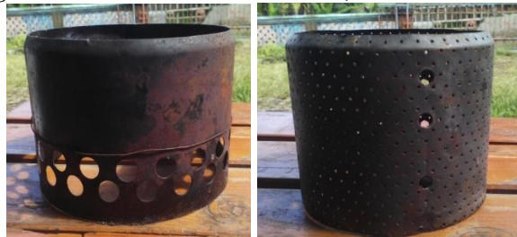
Figure 5. Air inlet at the stove wall, before modification
