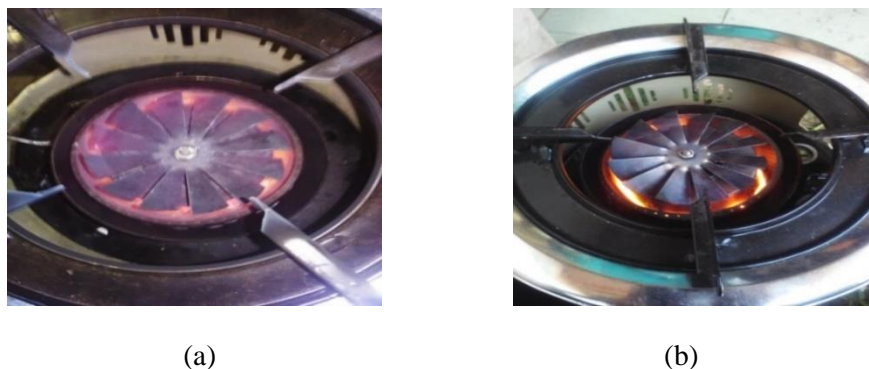
Figure 11. Flame color (a) before modification, and (b) after modification
