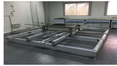
Figure 4. The test frame for installing photovoltaic module.
