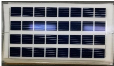
Figure 3. Monocrystalline silicon double glass photovoltaic module.
